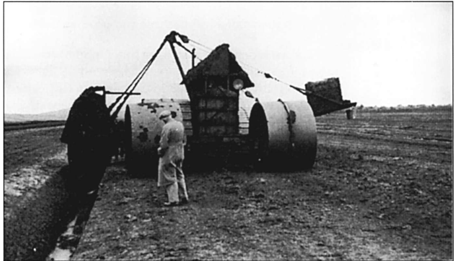
Figure 4.14: C.S.V. Smith OBE of Garretts, at Lullymore in 1947 during the redesign period of the machines for milled peat Production. Smith was a bog machine designer With Garretts, who were responsible for the design of the machines provided to Lullymore in 1935 and 1947, and for Boora, Derrygreenagh and Blackwater in 1952. Note the flat Wheels and tracks, Which ensure a flat surface on the fields harveted for milled peat. (Photograph J. Martin).
